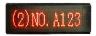
Shape made of injection molding, beautiful appearance, convenient installation, suitable for different parts of the installation. High brightness red LED display, resolution is 16\*96(16 dot-matrix 12 characters LED) Power supply by inner Switch Power DC 5V
